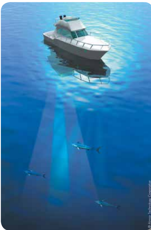
This image demonstrates the difference in beamwidth of 50kHz and 200kHz. In this example, the wider 50kHz beam will show returns for fish that the narrow 200kHz beam would have missed.
